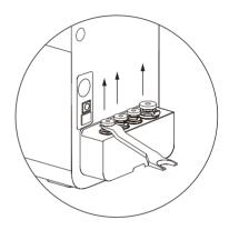
b. Connect the water inlet and the three-way ball valve.
